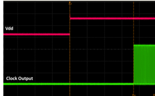
Figure 16. Startup Waveform vs. Vdd
